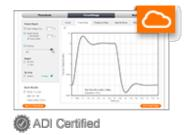
Use Photodiode Wizard to design a transimpedance amplifier circuit to interface with a photodiode. Select a photodiode from the library included in the tool, or enter custom photodiode specifications. Quickly observe tradeoffs between Bandwidth, Peaking (Q), and ENOB/SNR. Modify circuit parameters, and immediately see results in plots for pulse response, frequency response, and noise gain.
