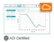
Use the Analog Filter Wizard to design low-pass, high-pass, or band-pass filters with actual op amps in minutes. As you progress through the design process, you can observe the characteristics of your filter design from ideal specifications to real world circuit behavior. Quickly evaluate the tradeoffs in op amp specifications - including gain-bandwidth, noise, and supply current - to determine the best filter design for your requirements.
