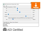
This tool aides in determining the proper pullup resistor size for a 1-Wire system by taking into consideration the system's supply voltage, tolerance, along with parameters for both the host and target.
